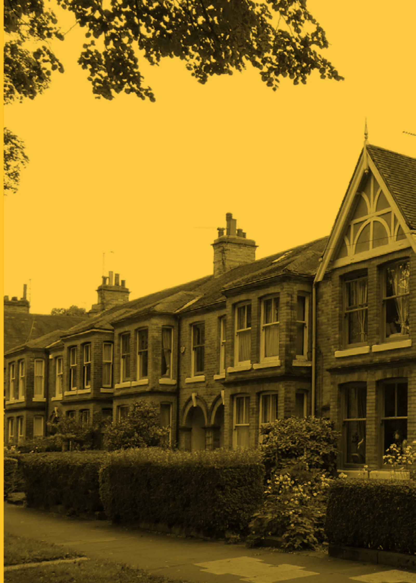
Fig 23: The Avenues, Hull. Positive street frontages are achieved through large bay windows, set back and articulated front doors, front gardens, generous soft landscape, wide pavements and mature trees.
