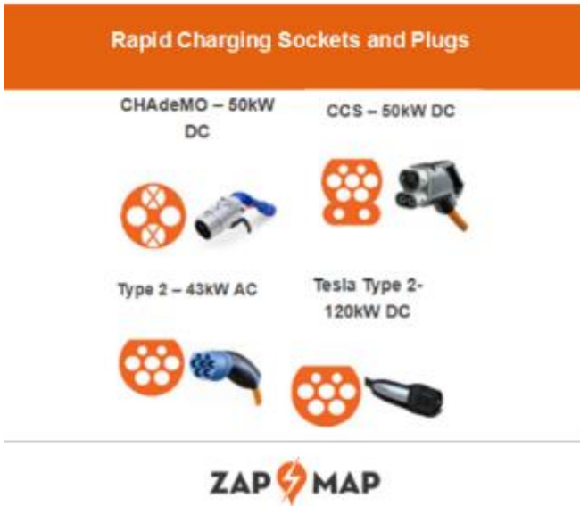
Figure 3- 3: Sockets and plugs for rapid and high-power charging in UK
