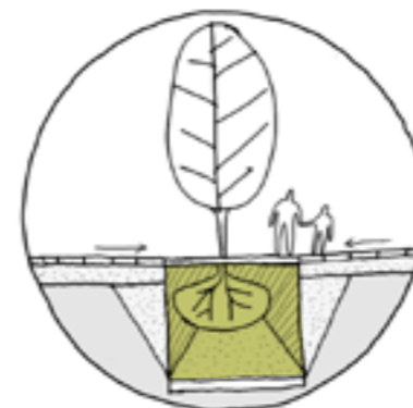
Tree pits provide on-site attenuation of run off water
