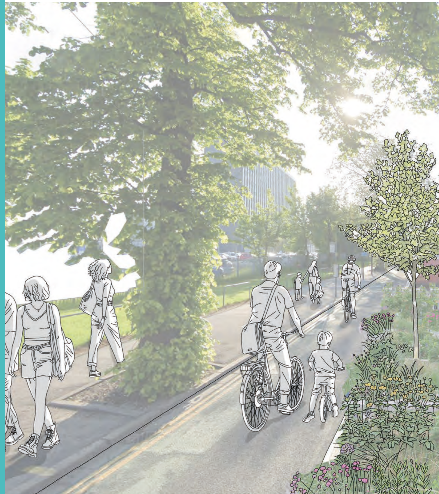
Figure 3.1: Concept image exploring the improvement of footpaths and cycleways along Anlaby Road, and incorporating landscape (which doubles as a sustainable urban drainage system for rainwater) as a buffer between pedestrians, cyclists and road vehicles.
