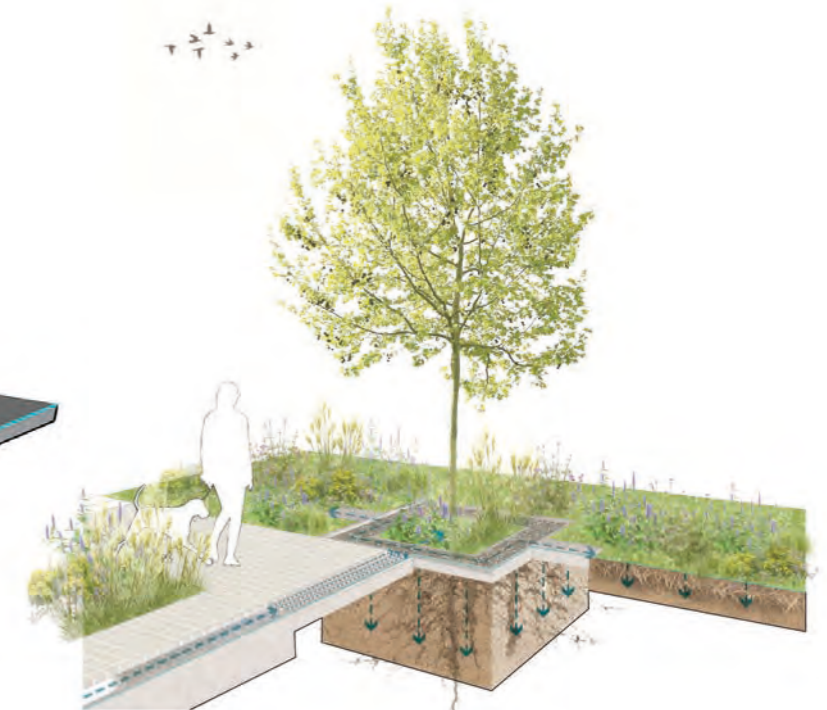
2. Streetscape SuDS Solution - Tree pits specifically designed to receive and manage storm-water, this alongside planted areas which supplement the water capacity held within the pits.
