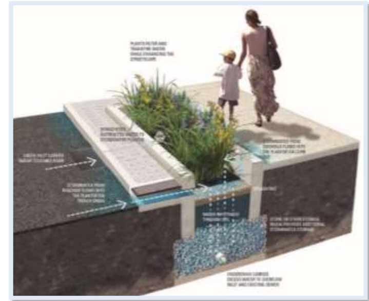
Figure 58 - Drawing showing the principle of storm water drainage system integrated into the soft landscape treatment (Water Phila, 2023)
