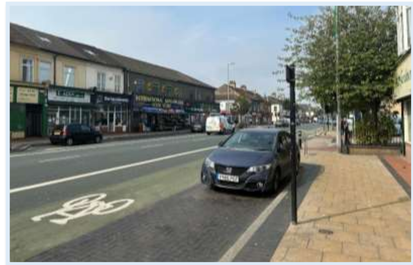
Figure 30 - Photograph of the existing cycle lane showing the conflict with the car parking / service bays
